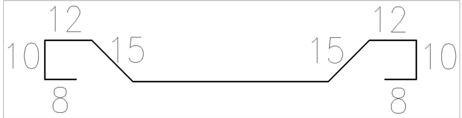
Length: 450.0000 MM    Width: 380.0000 MM    Thickness: 0.    Material: Cold plate    Initial value of axis C: 0    Show advanced actions     Display compensation parameters    Template selection: Default
