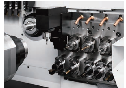
U12B (Rear tool post incorporating Y axis)
