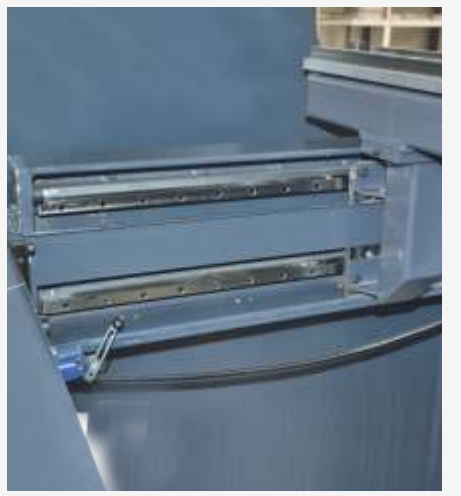
Linear Guided Stronger Back Gauge X Movement
