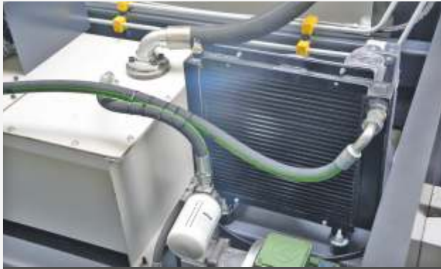
Hydraulic Oil Cooling System
