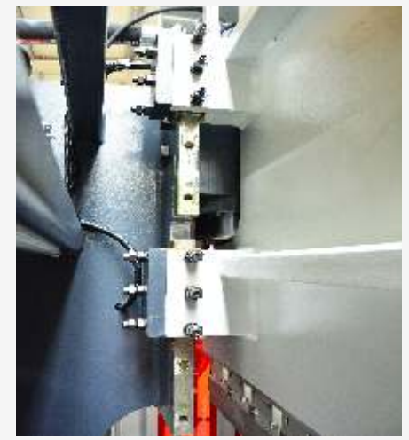
Stronger Beam Guiding System to stable the beam
