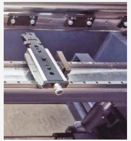
Double Linear Guided Stronger Back Gauges
