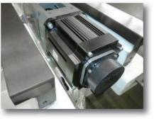
16mm fine pitch ballscrews in combination with 67 million pulse encoder technology provide a new degree of contouring accuracy - at least 4x of this technology.
