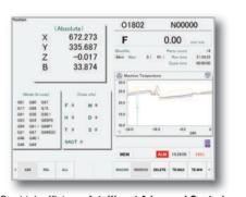
Our high efficiency Intelligent Advanced Control System (IAC) consists of a series of strategically located sensors and machine efficiency monitors that work to keep component growth due to machining heat build-up to less than ±5 microns (±0.0002").
