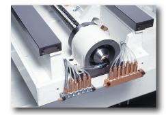
Ballscrew temperature is precisely controlled by an internal ballscrew cooling system. This eliminates thermal growth and promotes rigidity assuring peak machining precision even under prolonged heavy cutting conditions.
