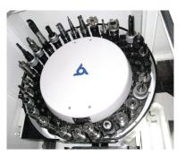
**Tool Handling** Efficient tool handling slashes idle time to maximize machining profit. The Mycenter-3020G ATC uses a memory-random tool selection system for smooth idle-free tool changes. Its generous 30 tool ATC enhances machining capability.
