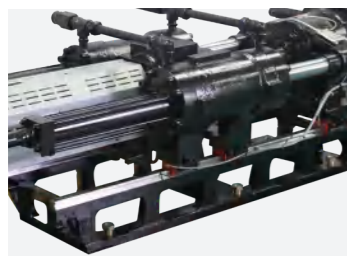
Injection unit support with linear guide rails
