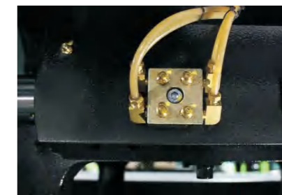
User-friendly design: movable hopper rails (60T-320T) Centralized lubrication module
