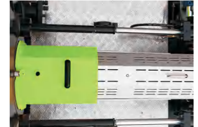
Horizontal double-carriage design
