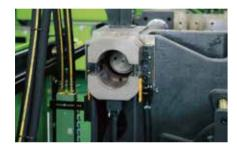
Impact-proof synchronized lock nut mechanism
